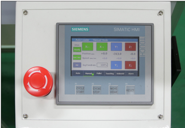
Convenient mobile operator's panel for loader setup
