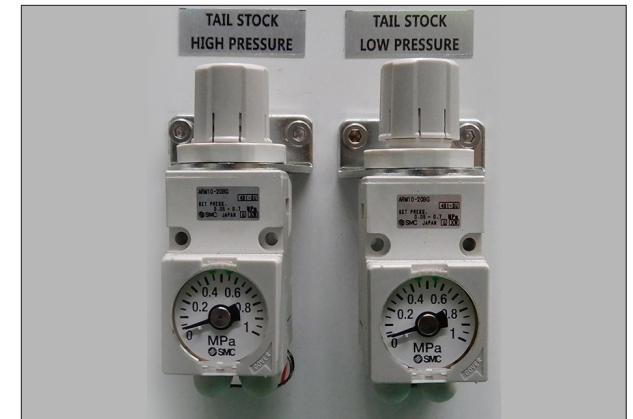
Low and high pressure adjustable tailstock for automatic lens centering
