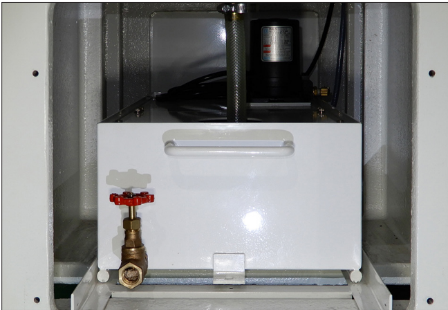
Coolant pump and tank mounted underneath the machine body
